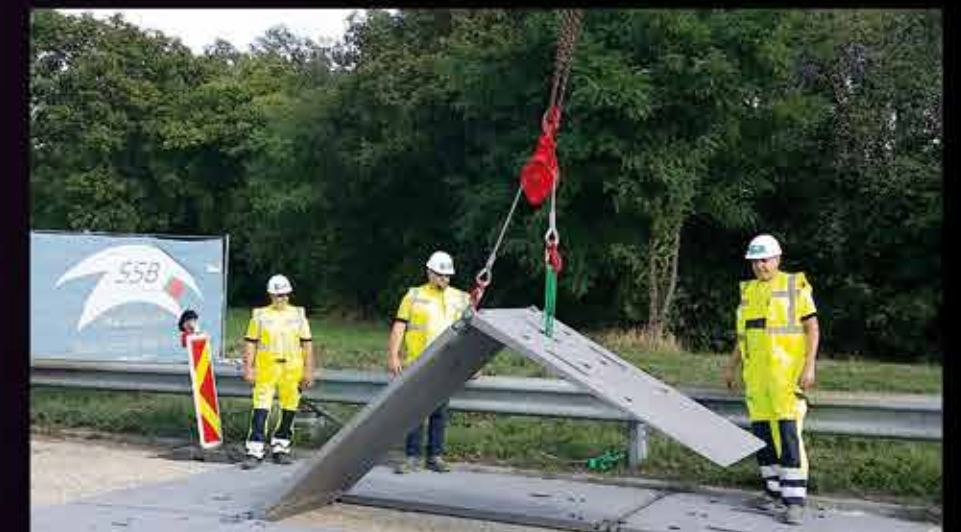
Scrutinising eyes during a function test of an MMBS element.
